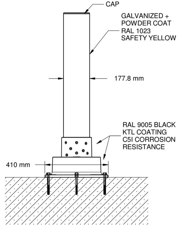
\* MINIMUM FOUNDATION DEPENDS ON LOCAL SOIL CONDITIONS, WEATHER & ENG. REQ'TS
